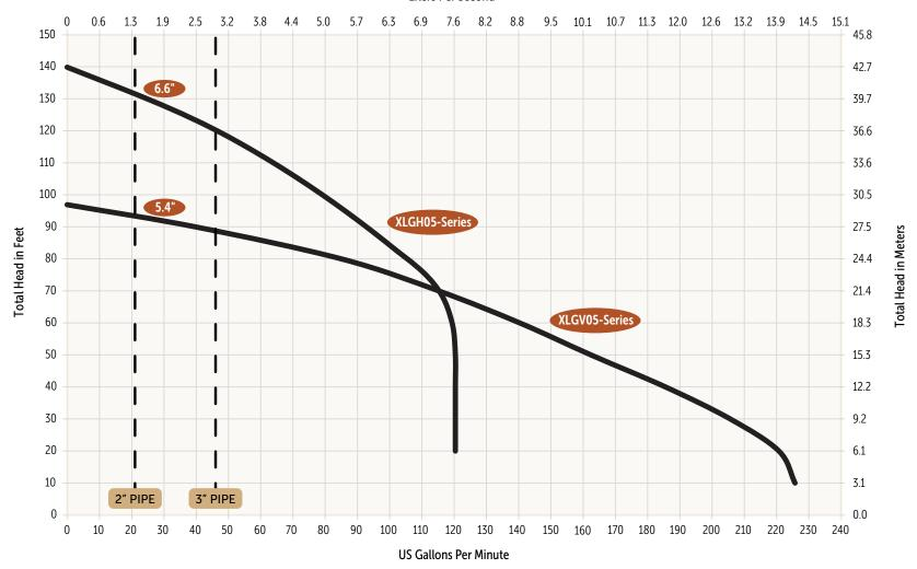
Pumps must operate within the proper range shown on the performance chart. It is the responsibility of the end user to ensure this requirement is met. Pumps operating outside the recommended range are prone to damage, excessive vibration, cavitation, poor efficiency, and may exceed nameplate amperage.
